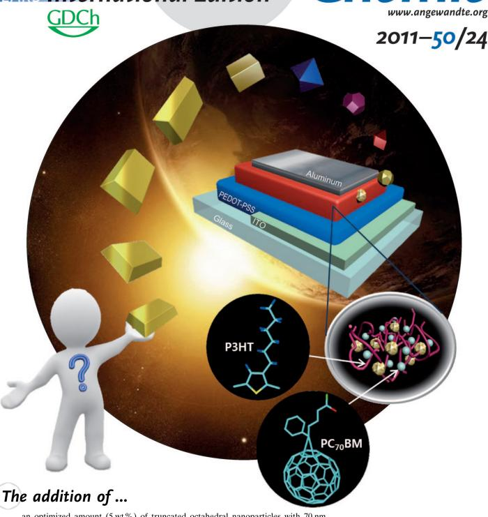
... an optimized amount (5 wt%) of truncated octahedral nanoparticles with 70 nm diameter leads to an increase in power conversion efficiency in bulk heterojunction photovoltaic cells. In their Communication on page 5519 ff., J. H. Park, O O. Park, A. J. Heeger, et al. describe the fabrication of such solar cells from a variety of donor polymers and  $PC_{70}BM$  as acceptor.
